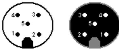
Fig. 3: Pin code: Connection plug / socket
