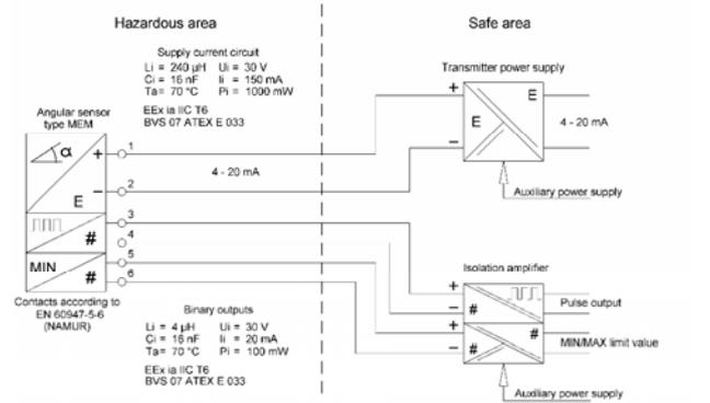
Terminal diagram for measuring transducer HART with 4–20 mA output and 2 limit contacts
