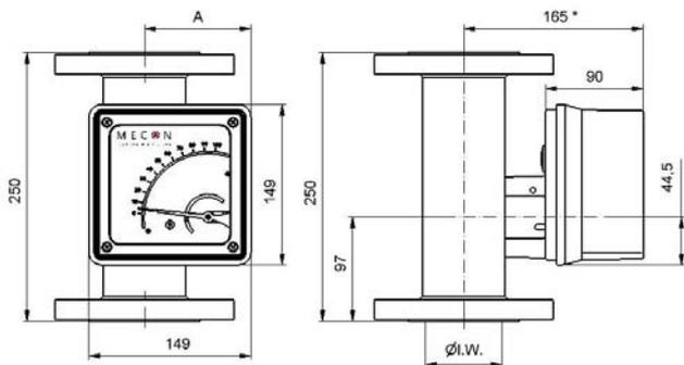
Fig. 3 Housing of display made of aluminium
