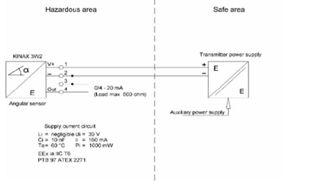
Terminal diagram for measuring transducer KINAX 2W2 with output 4–20 mA in 2-conductor technology
