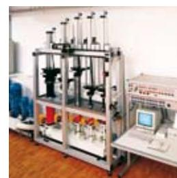
Each KRAL Volumeter is tested and calibrated on our in-house test bed. Depending on customer requirements, we perform either a factory calibration or a calibration in compliance to ÖKD (Austrian Calibration Service).
