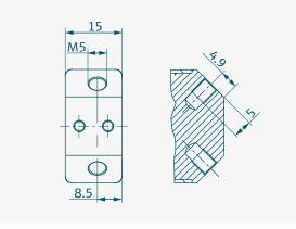
Dimensions in mm for fluid installation
