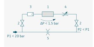
Installation example: 1 = Density sensor; 2 = Valve; 3 = Filter; 4 = Flow restrictor; 5 = Orifice Making the electrical connections for the density sensor
