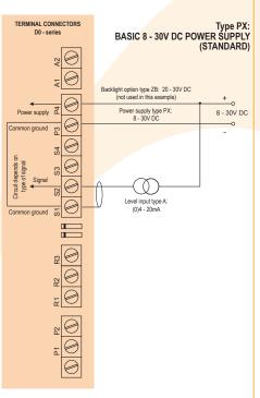
\* Sensor supply voltage for analog sensor type A / U: Terminal S3: not available.
