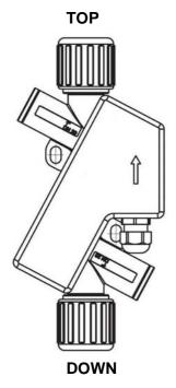
Fig. 2: Installation position of Flowmax 400i
