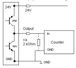
Fig. 6: Connecting output Q2 to counter
