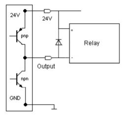
Fig. 5: Connecting output Q1 to relay
