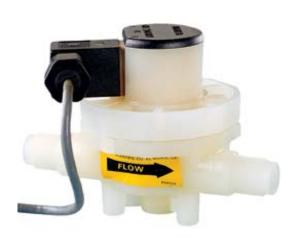
The Signet 2507 Mini Flow Rotor Sensor contains a free-running rotor that is driven by the fluid flow. Within the given measurement range, the rotational speed of the rotor is proportional to the fluid flow rate.
