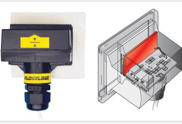
The general purpose non-intrusive capacitance level switch provides reliable liquid level detection of water based conductive liquids with non-coating and/or scaling characteristics with a 1A relay output. Media examples include hydrochloric, sulfuric acid and water. The liquid level sensor is bracket mounted on the exterior wall of non-metallic tanks and applied as a high level alarm or low level alarm.
