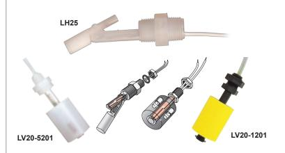
Offered in vertical and horizontal configurations, the general purpose mini-float level switches provide reliable liquid level detection of clean water and chemical solutions with a 15VA or 30VA reed switch output. Media examples include water and sulfuric acid. The polypropylene or PVDF liquid level sensors are mounted vertically inside the tank or horizontally through the tank wall as a high level alarm or low level alarm.
