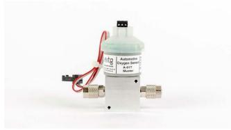
The O2.sens from Wi.Tec is based on an electrochemical process. In this process, a chemical reaction takes place with the oxygen to be measured and a liquid electrolyte. In this reaction, 4 electrons are released per oxygen molecule. The resulting sensor current IM or the measurement voltage UM increases proportionally with the number of reacting O2 molecules. This results in a sensor characteristic that increases linearly with increasing O2 concentration.
