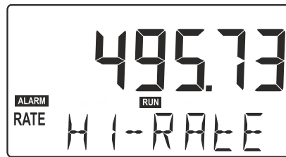
Fig. 5: Example of a flowrate alarm.
