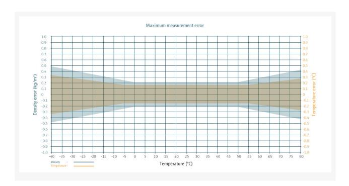
*Max. measurement deviation: Density and temperature*
