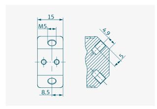
Dimensions in mm for fluid installation
