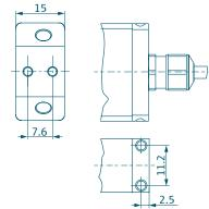
Dimensions in mm for mechanical fastening
