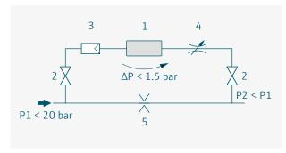
Installation example: 1 = Viscosity sensor; 2 = Valve; 3 = Filter; 4 = Flow restrictor; 5 = Orifice
